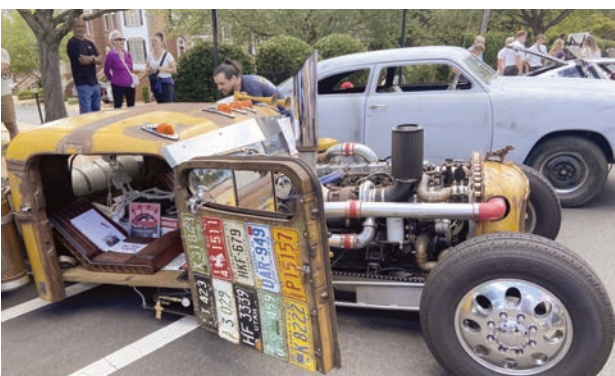
Adam Alami looking at this creative Mack "rat" rod made from a 1954 Mack truck, with a Dodge chassis, 1932 Ford front end and a 1990 diesel engine.
